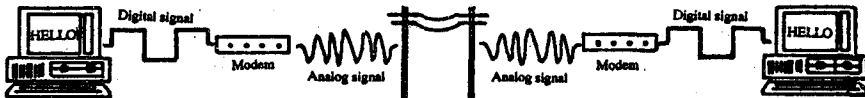
Fig. 2.2 : The basic elements that make up a communications link between two computer systems
